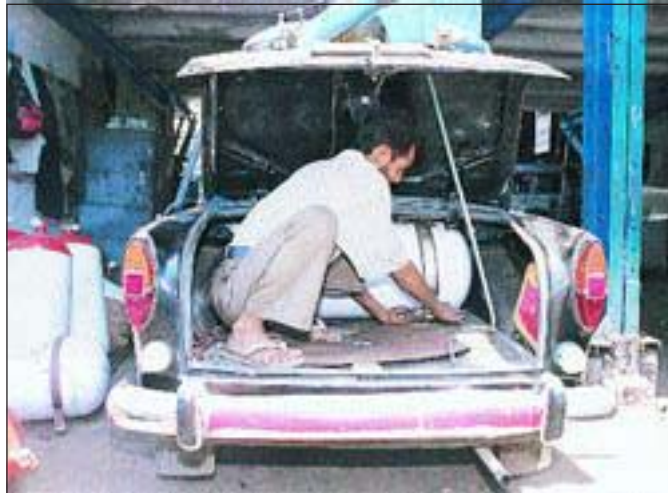
A taxi being converted to use CNG
